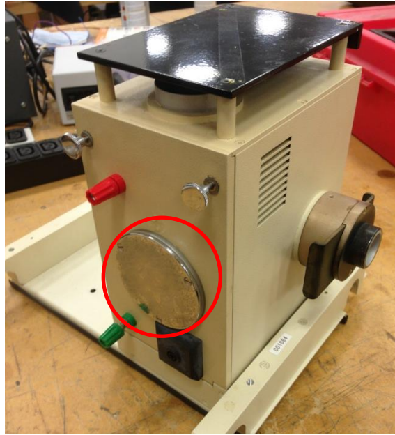
Figure 5.4 - Location of cover plate for lamp alignment mirror.
