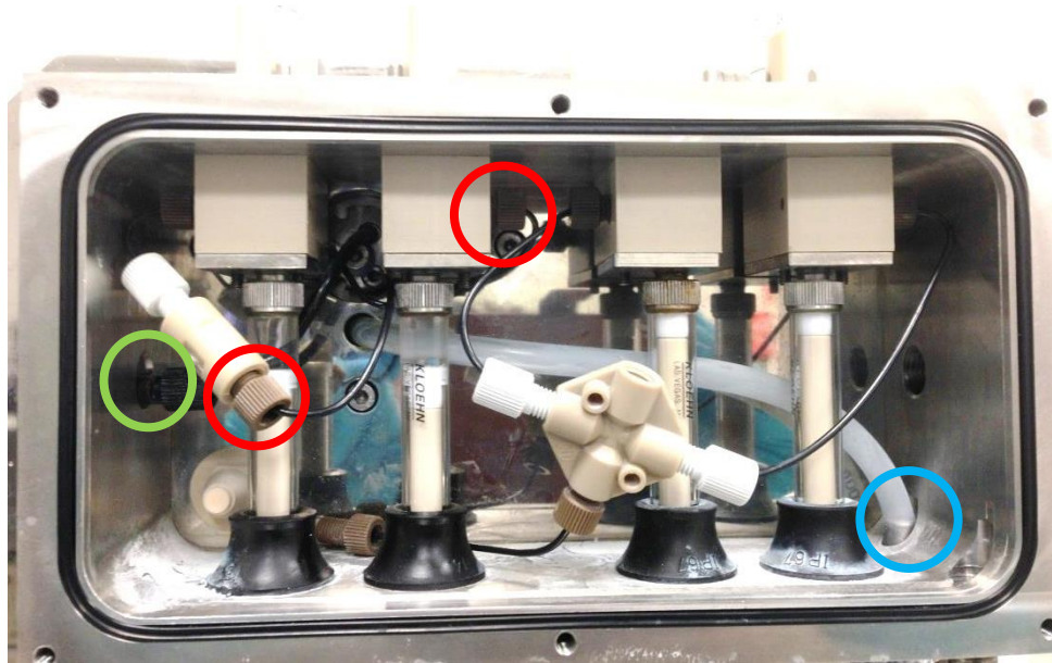
Figure 3.31 - Location of tubes to disconnect prior to water bath removal
