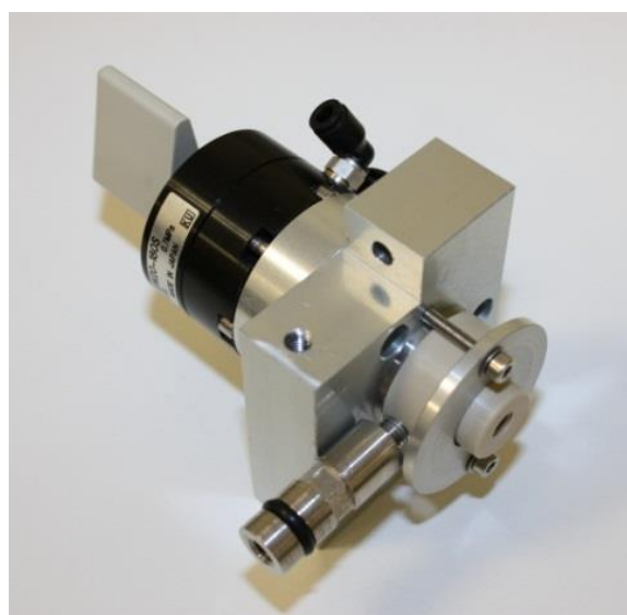
Figure 3.24 - A correctly assembled stop valve actuator
