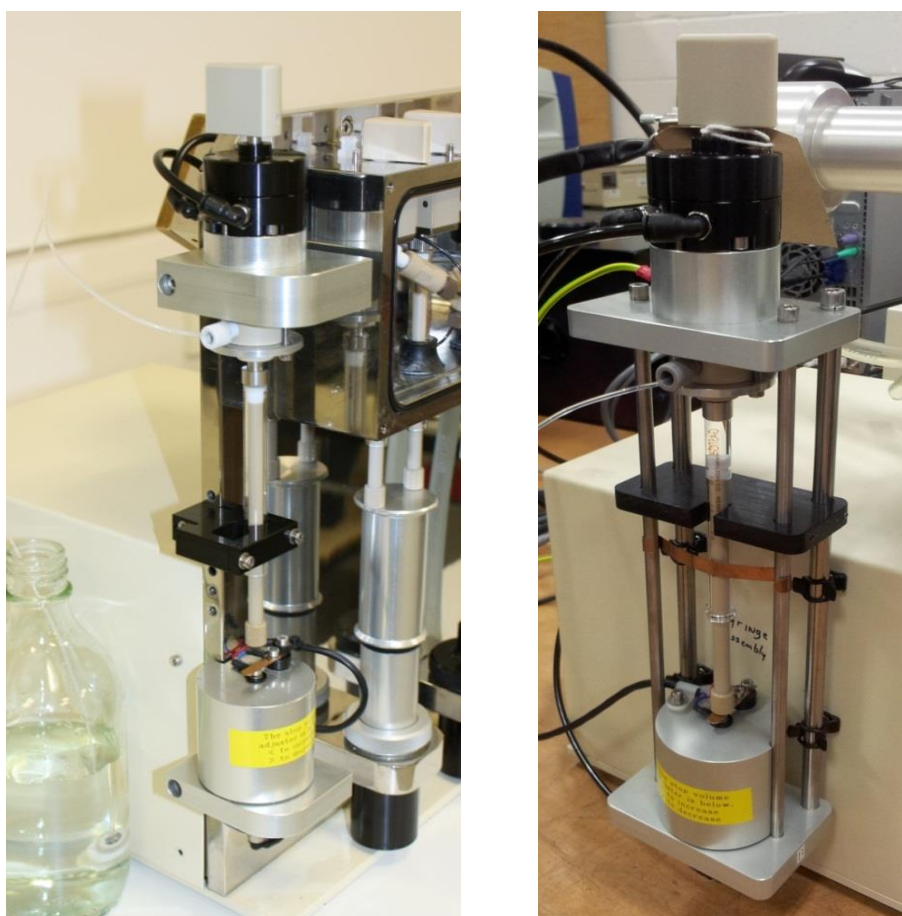
Figure 3.16 - Left: SX20 autostop assembly, Right: Older SX18 and SX19 autostop assembly
