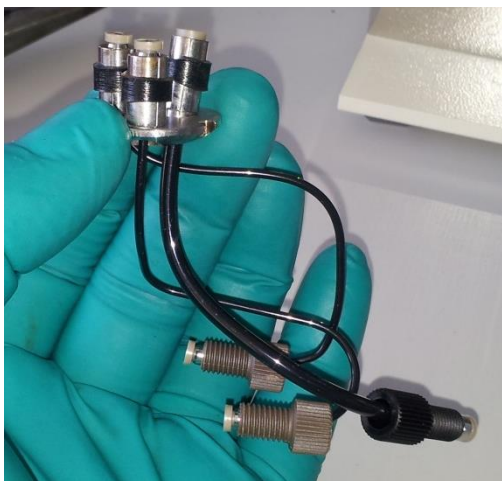
Figure 3.35 – An assembled, new and clean flow tube assembly
