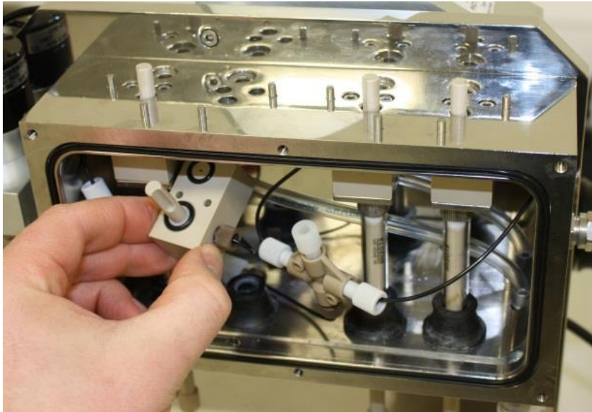
Figure 3.14 - Dropping a drive valve
