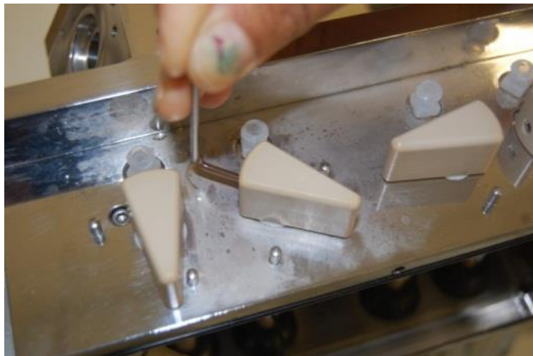
Figure 3.11 - Location of drive valve knob grub screws
