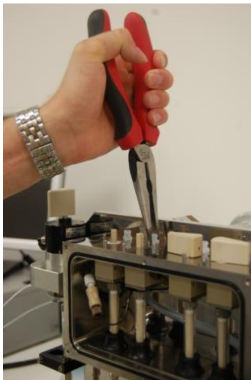
Figure 3.12 - Removing the luer fittings
