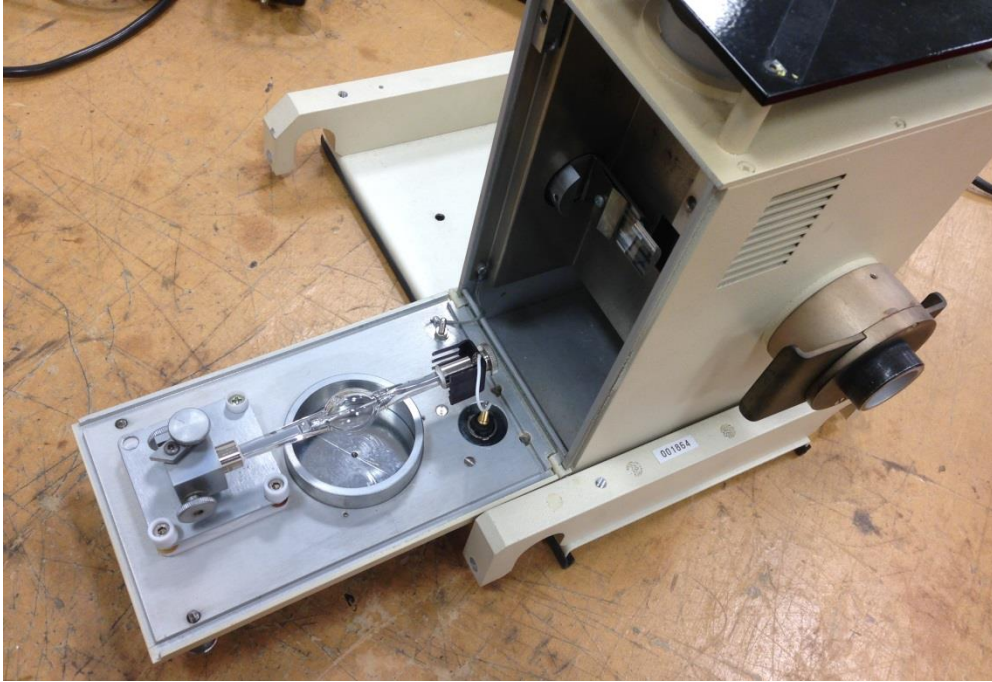
Figure 5.2 - Opening the cream lamp housing
