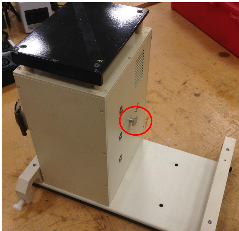
Figure 5.6 - Location of mirror adjuster on cream lamp housing
