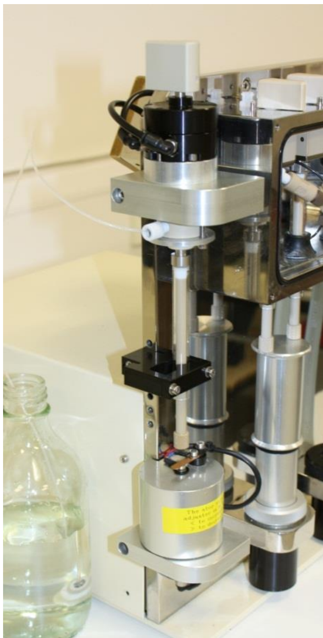
Figure 3.26 - A complete autostop assembly (no brake shown)
