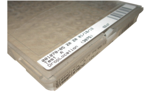
Figure 4-13. LCP Plate Adaptor.
