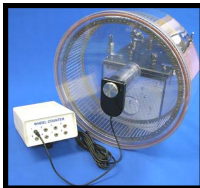
Rat 30cm Running Wheel with Rotation Detection Interface
