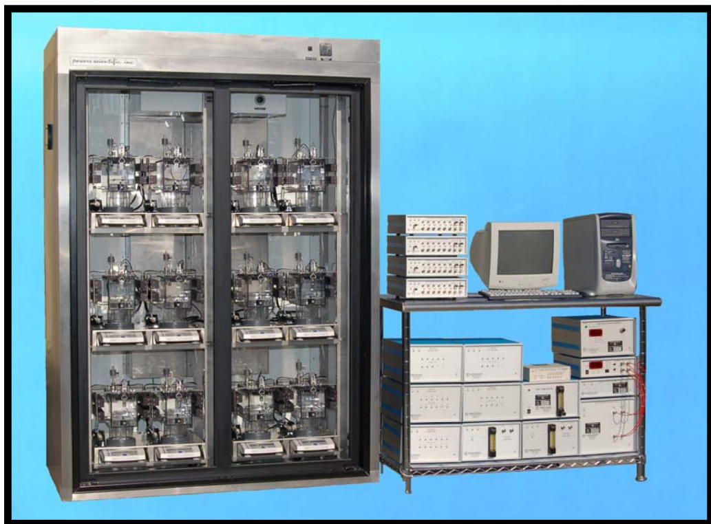
12-Chamber Mouse System with Calorimetry, Activity, Feeding and Drinking Monitoring
