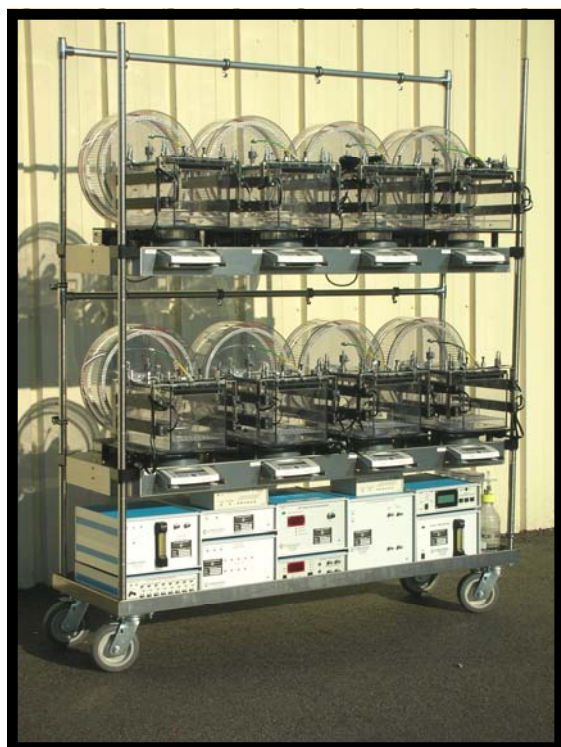
8-Station Rat Oxymax/CLAMS with 30cm Running Wheels
