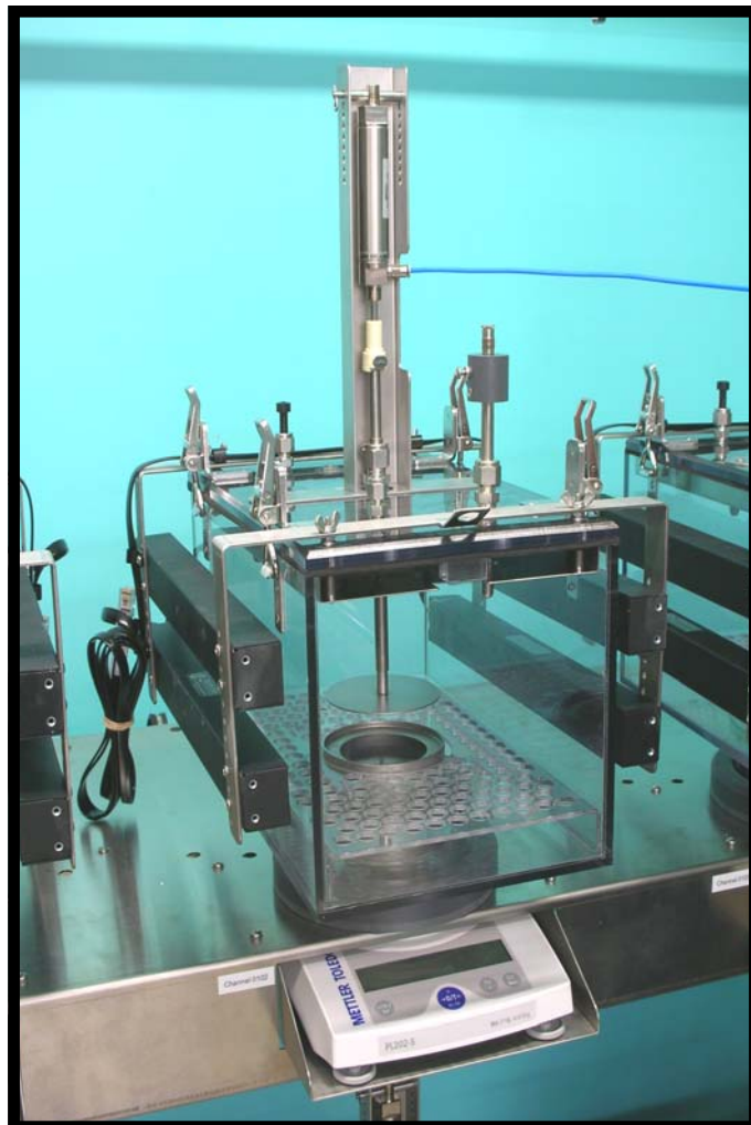
Custom Automated Food Hopper Access Control for Center Feeder Rat Chamber
